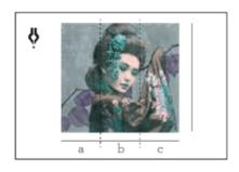
On the first and on the last roll 2 red lines indicate the exceeding material. These lines are necessary to correctly locate the subject on the wall. 5 cm on the top and 5 cm on the bottom of the rolls will have to be removed during the application phase.
