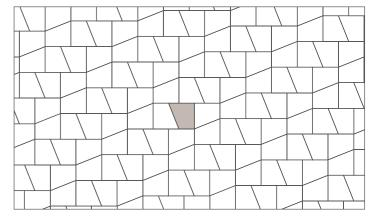
These elements are milled with groove profiles on four sides. They interlock by means of solid wood loose tongues supplied with the material.
