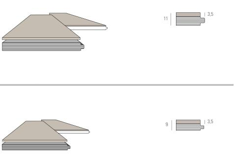
All products in the Classica range are compatible with heating and cooling underfloor systems provided they are installed with the glue down method and the instructions on operating temperature and humidity are strictly complied with.
