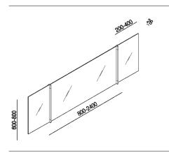
Modular rectangular mirror with visible hinges in polished stainless steel, with height 60 (23" 5/8). Divided into three elements with polished edges and safety film.
