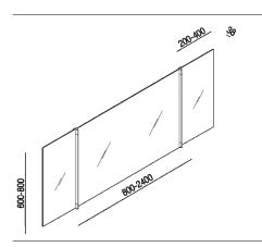
Modular rectangular mirror with visible hinges in polished stainless steel, with height 80 cm (31" 1/2). Divided into three elements with polished edges and safety film.
