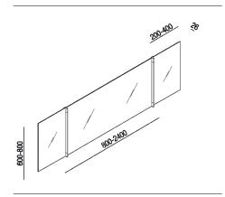
Modular rectangular mirror with visible hinges in polished stainless steel, with height 60 cm (23" 5/8). Divided into three elements with polished edges and safety film. Central element with standard or custom measures; two-sided adjustable lateral elements in different shapes and widths. Optional switch always positioned at the centre of the bottom edge. The mirror is fixed to the wall by means of screws and wall plugs.
