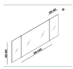
Modular rectangular mirror with visible hinges in polished stainless steel, with height 80 cm (31" 1/2). Divided into three elements with polished edges and safety film. Central element with standard or custom measures; two-sided adjustable lateral elements in different shapes and widths. Optional switch always positioned at the centre of the bottom edge. The mirror is fixed to the wall by means of screws and wall plugs.
