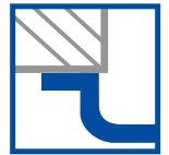
Countertop extends over the edge of the sink.
