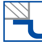
Countertop edge sits back from the edge of the sink, exposing the sink rim, typical 1/8".
